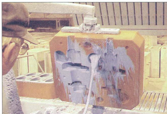
Flow coating is a method of applying a refractory coating that can be described as "wetting the mold with a garden hose at low pressure." With the flow coating method, the mold/core is maneuvered so it is at an angle in front of the operator. Even under low pressure, the coating can penetrate the sand and let the excess run-off.
