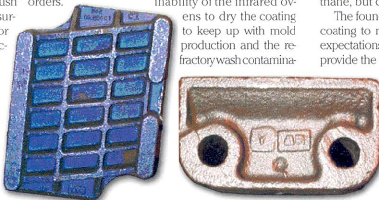
Fig. 2. Flow coating results in a smoother looking surface finish as shown on this as-cast steel casting (l) as compared to the casting (r) that was spray coated. Flow coating also eliminates burn-in and burn-on sand defects, which in turn reduces machining costs.
